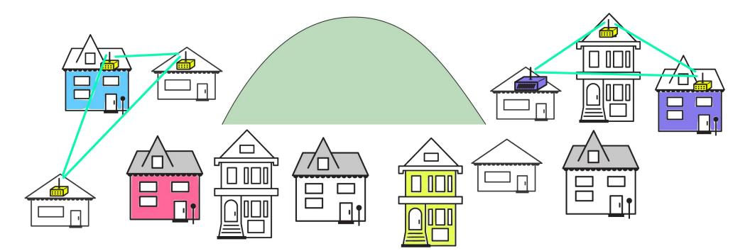
**Problem 7:** The number of wireless signals in your building causes slow connections on the mesh.
