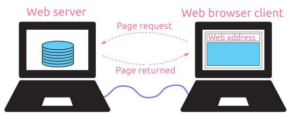
Most requests and content delivery on networks are similar to, or are based on, a client to server relationship. On a network, the server can be located almost anywhere, and if the client has the address, it can access the content on the server.
