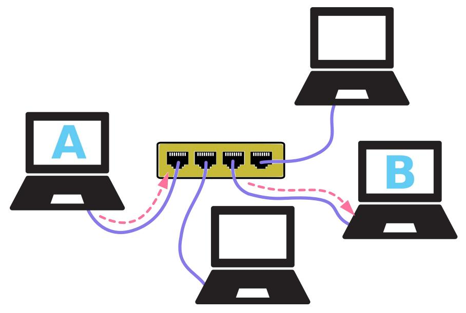
Switches do have a limitation though—they only know about the addresses of equipment that is plugged directly into them. So, you can only send messages to a small number of devices—however many ports the switch has! If you need to send a message to a computer on another network, it will need to be sent through a router, which we discuss next.
